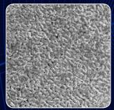
Battery separator material "Celgard" with 2.5 microns of Lithium (x2000).
