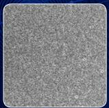
17 microns thick Copper foil with 19 microns of Lithium (x 500).
