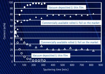
XPS analysis of Li metal Comparison of vacuum deposited Li thin film and rolling Li foil
