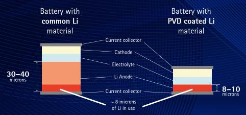
Comparison of batteries with conventional rolling and PVD coated Li
